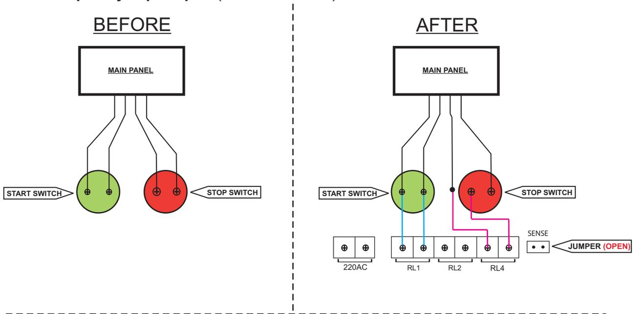
Control Panel with START and STOP switch and START switch has four terminals (connections) behind it.
