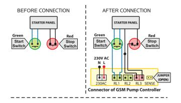
Control Panel with START and STOP switch and START switch has four terminals (connections) behind it.
